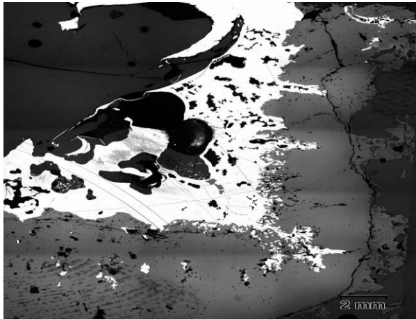
Fig.4.3. Case of P.M.C.M. - V.L.C.S interaction: 1 - steel; 2 – penetrated ceramic mixture
